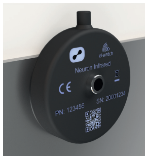
Place elevated with distance to fixed objects
