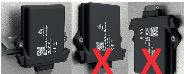
Gateway with mounting kit. Do not mount directly on wall or other structures. Connect the power plug (from the Neuron PSU or Neuron Power Cable) to the power inlet on the gateway. The power inlet is the lower part of the gateway in the picture on the left above.
